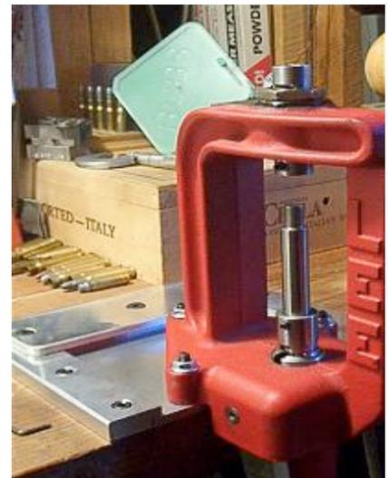
Check that your copper strip slides through easily from end to end, then insert your strip, and cut your disks. I love the LEE Classic Cast because there is ample headroom, and it's easy to adjust your arm where the leverage is comfortable. Level horizontal is about where I like the arm.
