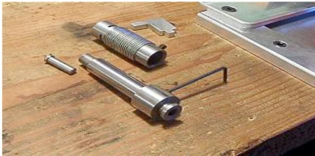
Thread the upper 7/8-14 female disk cutting housing in your press with enough threads on top to get a nut on. **Carefully raise the male die up into the female housing and check for alignment-** **\*\*If the male die does not clear the internal female cutter die, rotate threaded housing to correct, then tighten the nut-recheck.** May need to rotate male die also **\*\*make sure the housing set screw is backed out of the way\*\*** Snug tight is fine.
