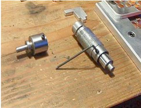
Set the ejector pin in the lower female forming die, and set the ram ejector arm in the ram's primer slot. Install the female forming die in the shell holder. **\*\*make sure the lower female forming die set screw is backed out of the way\*\***
