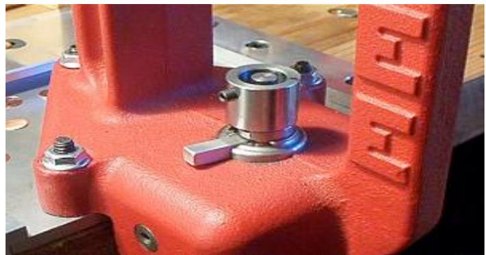
Drop a disk into the forming die. **\*\*The best way is to just drop it in\*\*** Don't try to set it in there. If it doesn't fall dead center with the drop (most of the time it does), bring the ram up and just "kiss" the disk. 99 times out of 100, it will bump it in it's seat.
