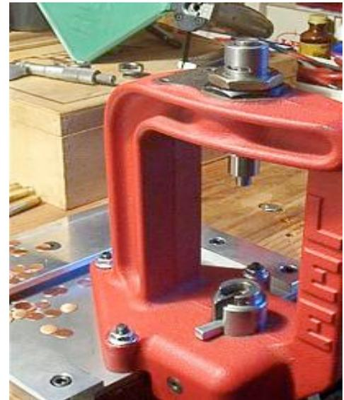
Pic shows Lower female forming die with ejector pin, and ram ejector arm in press. The ejector pin's head is also the base that the check is formed against, providing a solid flat surface in the forming die.
