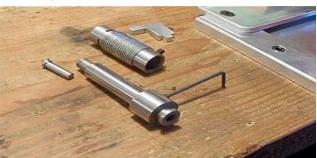
Thread the upper 7/8-14 female disk cutting housing in your press with enough threads on top to get a nut on. Carefully raise the male die up into the female housing and check for alignment-\*\*If the male die does no clear the internal female cutter die, rotate threaded housing to correct, then tighten the nut-recheck. May need to rotate male die also \*\*make sure the housing set screw is backed out of the way\*\* Snug tight is fine.
