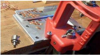
Pic shows Lower female forming die with ejector pin, and ram ejector arm in press. The ejector pin's head is also the base that the check is formed against, providing a solid flat surface in the forming die.
