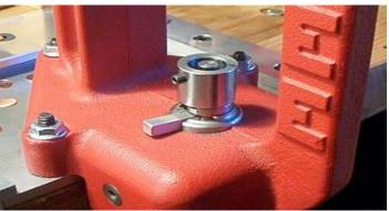
Drop a disk into the forming die. \*\*The best way is to just drop it in\*\* Don't try to set it in there. If it doesn't fall dead center with the drop (most of the time it does), bring the ram up and just "kiss" the disk. 99 times out of 100, it will bump it in it's seat.
