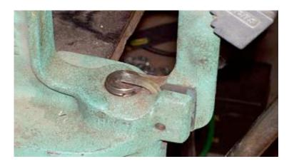
**Sharpening** The Checkmaker male disk cutting die is hardened steel and fortunately VERY simple to sharpen unlike a conventional hole punch. Anyone can do it in a minute. You need to purchase an EZE-LAP flat diamond hone sharpener. I've bought these on sale for around \$7 here:
