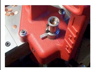
Set the ejector pin in the lower female forming die, and set the ram ejector arm in the ram's primer slot. Install the female forming die in the shell holder. \*\*make sure the lower female forming die set screw is backed out of the way\*\*
